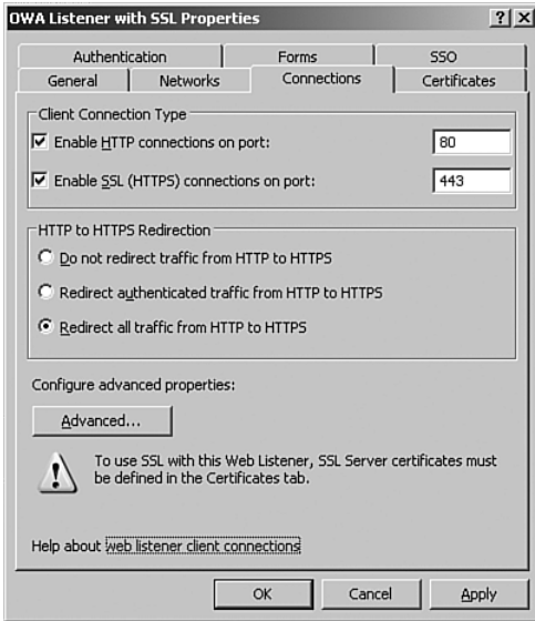
FIGURE 12.19 Automatically redirecting from HTTP to HTTPS.
