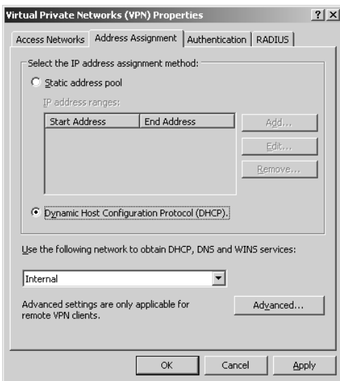
FIGURE 3.26 Enabling VPN client access.
