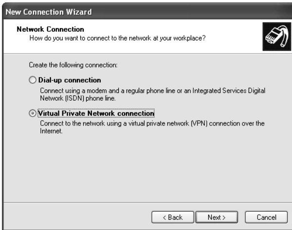
FIGURE 9.20 Configuring a Windows XP Professional client to use an L2TP VPN connection.
